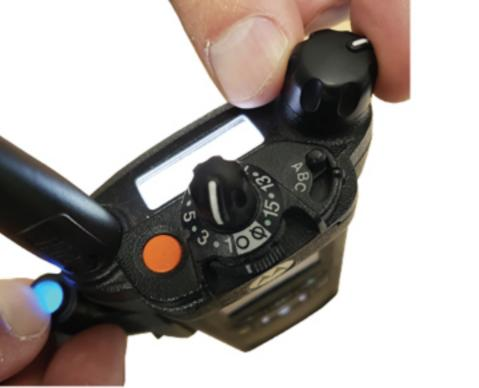
on the clear PTT button on the BT Adapter & turn the radio on at the same time. When BT Adapter is flashing Blue/Red release.
