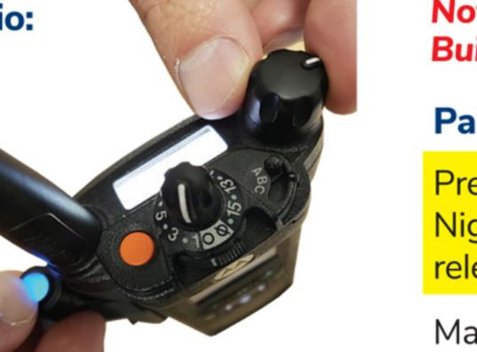
radio, press down on the clear PTT button on the BT Adapter & turn the radio on at the same time. When BT Adapter is flashing Blue/Red release. When both BT Adapter & Nighthawk are solid Blue for a moment both units are paired. No need to repeat the pairing process when this is achieved.
