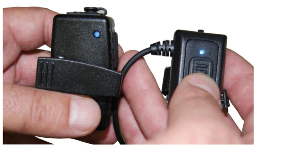
Disconnect the BTA from the USB. Upon doing so the BTA will power down. Short press the PTT button on the BTA until first LED appears then release. This will re-establish the link with the Bluetooth microphone.
