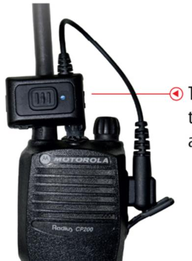
To secure the BTA dongle, wrap the Velcro strap around radio antennae.
