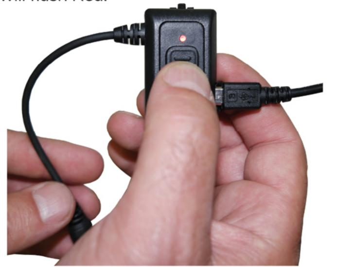
Press the PTT button on the BTA until LED is flashing Blue/Red then release.
