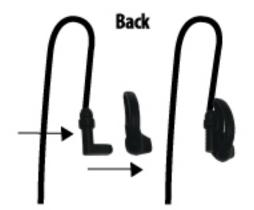
Curve of the wire should match the curve of the Fin Ultra™ ear tip.
