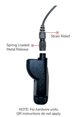
To connect, grab the cable from the connector with the fore finger & thumb on either side of the strain relief. When the connector falls into place, gently push down. Never force the connector into the adapter.
