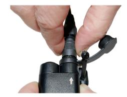
Note For Connecting XTS Adapter to the Radio: Attached bottom of the adapter first, pull back latch, press adapter against radio, release latch. Lock latch with screw.
