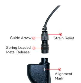
To connect, grab the cable from the connector with the fore finger & thumb on either side of the guide arrow. Align the guide arrow with the alignment mark on the radio adapter and gently push down.
