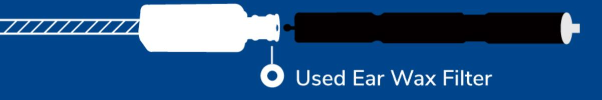
Re-insert a new white wax guard of the Filter Applicator into the speaker and gently pull.
