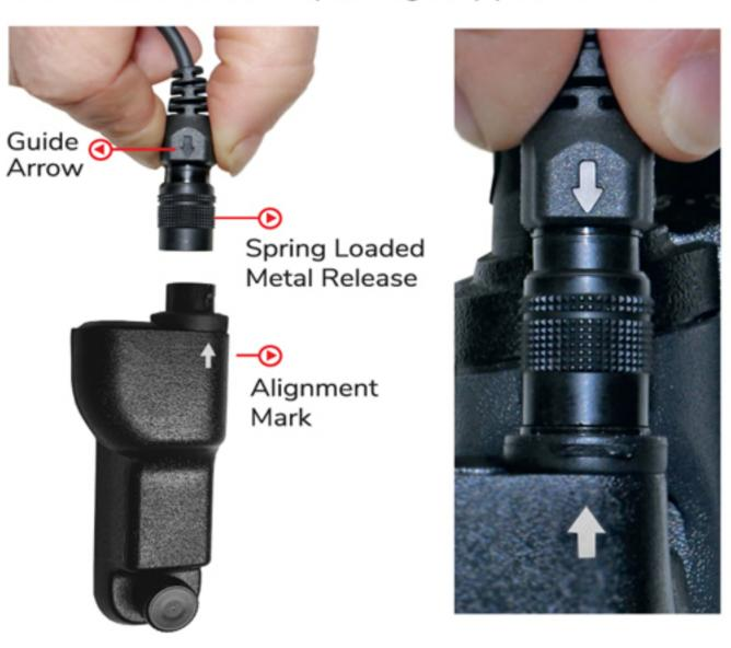
TO RELEASE, with the same two fingers grab the spring loaded metal release and pull up.
