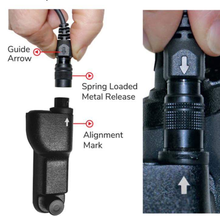
**To release,** with the same two fingers grab the spring loaded metal release and pull up.
