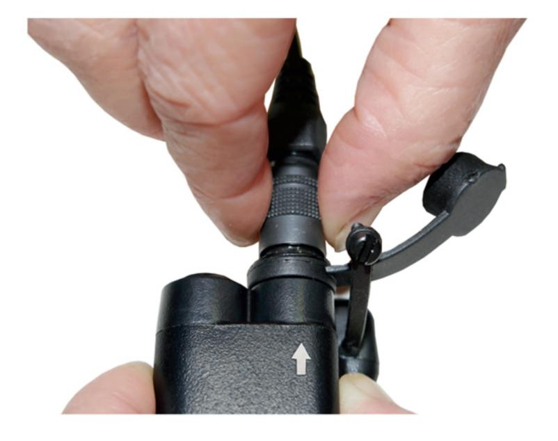
For Connecting XTS Adapter to the Radio: Attach bottom of the adapter first, pull back latch, press adapter against radio, release latch. Lock latch with screw.
